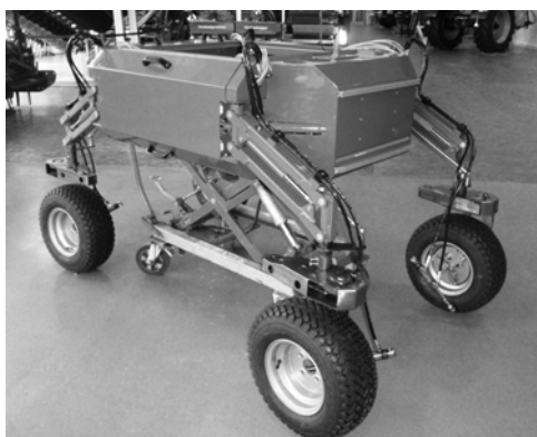
Figure 4. Autonomous vehicle BoniRob.
